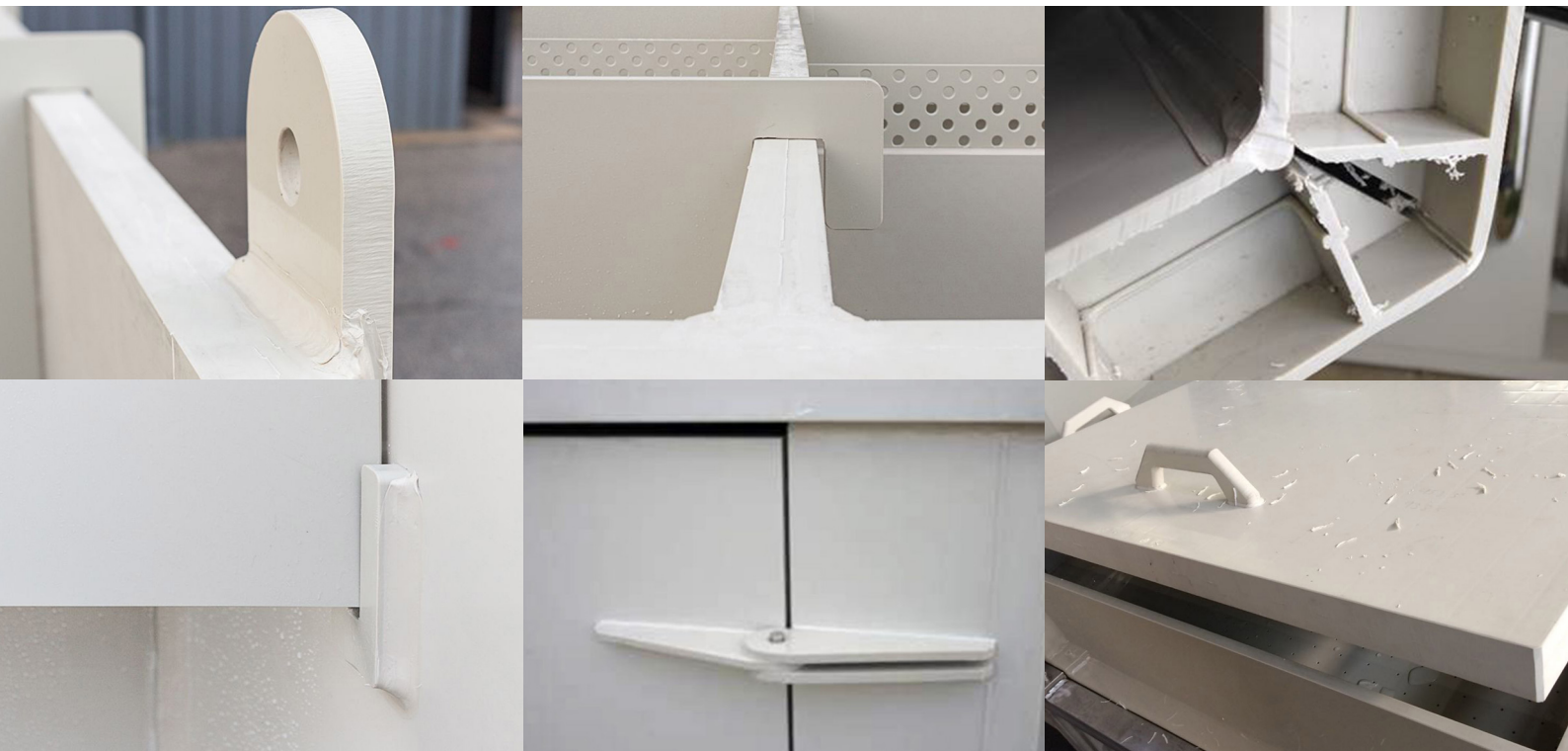
Fixing by plastic welding
