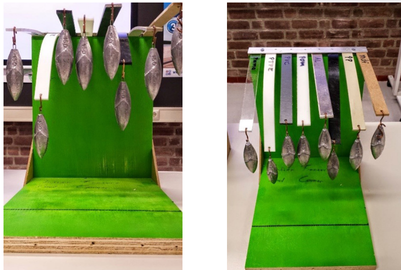
Experimental setup demonstrating creep.
